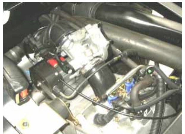
The Electric Actuator or throttle servo (2) is mounted to the frame below the drivers seat. An Actuator cable (3) connects the actuator to the CIU (see below).
