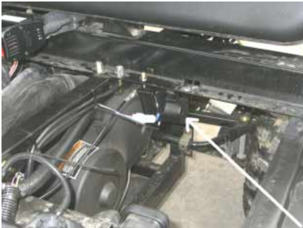
The Electric Actuator or throttle servo (2) is mounted to the frame below the drivers seat. An Actuator cable (3) connects the actuator to the CIU (see below).
