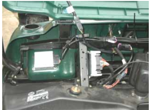
The Electric Actuator or throttle servo (2) is mounted to the frame below the drivers seat. An Actuator cable (3) connects the actuator to the CIU (see below).
